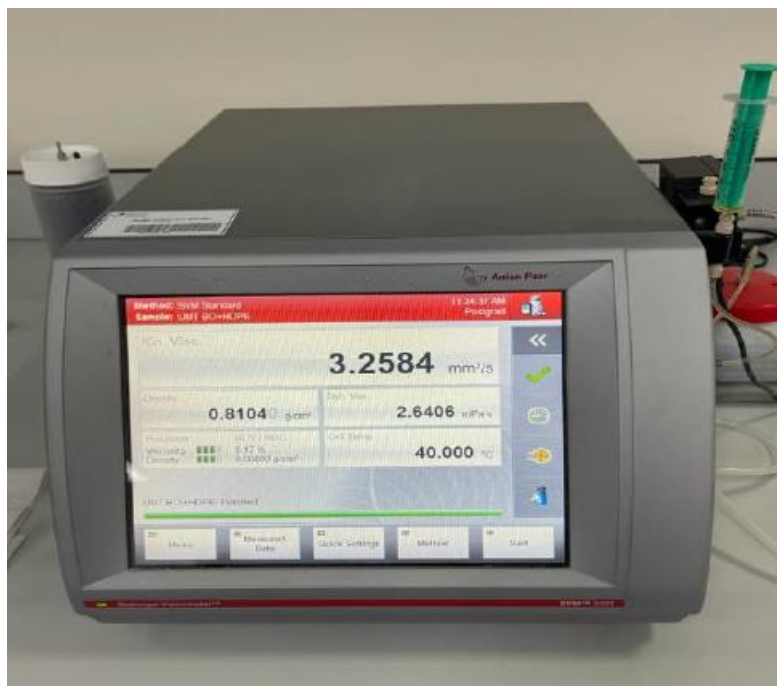
Figure 3.6 Portable kinematic viscometer (Anton Paar SVM 3001)
