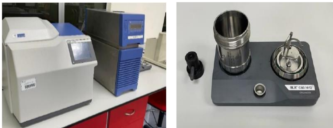
Figure 3.5 IKA Calorimeter C3000 and decomposition vessel with crucible
