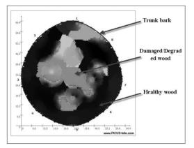
Figure 1: Example of Tomogram of a Palm Tree Internal Condition
