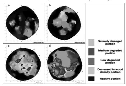
Figure 5 shows example of an tomogram of a palm with 0% damaged which was classified as a healthy tree. The palms show no external symptoms of BSR. As shown in Figure 6, four examples of palms were arranged respectively to their percentage of damage.
