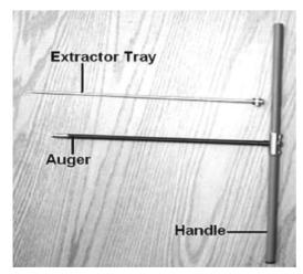
Figure 2: Increment Borer Device
