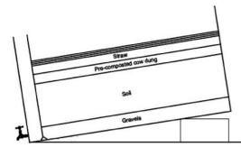
Figure 1: Illustration of Vermicomposting Leachate Reactor.
