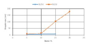
Fig. 6: Droplet size for 50:50 (\_\_\_\_) and 90/10 (.....) (mixed surfactant/1-But:MeAc) for  $H_2O/T$ ween 80/Span 20/1-Butanol/Methyl Acetate systems
