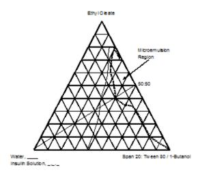
Fig. 4: Pseudoternary diagram for solvent/Span 20:Tween 80/1-Butanol/Ethyl oleate systems. The solvents are water, \_\_\_\_, and insulin solution, .....
