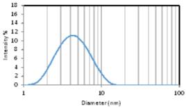
Fig. 5: The particle size distribution by DLS of microemulsion droplet described as intensity percent (%) at 5 weight % of water
