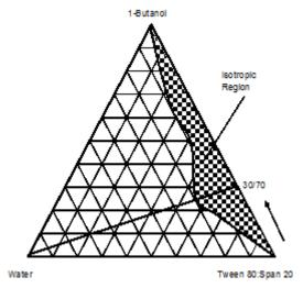
Fig. 2: Pseudoternary diagram for water/Tween 80:Span 20/1-Butanol systems
