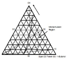
Fig. 3: Pseudoternary diagram for water/Span 20:Tween 80/1-Butanol /Oil systems (methyl acetate, \_\_\_\_ and ethyl oleate, ......)
