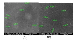
Figure 3 The particle sizes of  $TiO_2 NCs$  at different scan number (a) (1)  $TiO_2 NCs$  (b) (5)  $TiO_2 NCs$
