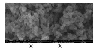
Figure 2 The surface morphologies of  $TiO_2$  NCs at different scan number (a) (1)  $TiO_2$  NCs (b) (5)  $TiO_2$  NCs
