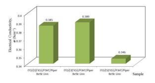
Figure 5 The electrical conductivity of hybrid solar cell at different scan numbers of  $\text{TiO}_2\,\text{NCs}$
