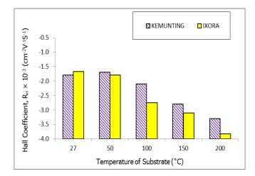
Figure 14 Variation of Hall coefficient with temperature of substrate for Bilayer Heterojunction OSCs
