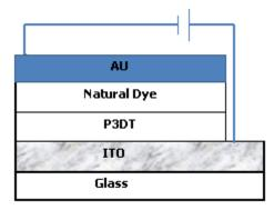
Figure 5 The structure of bilayer heterojunction of organic solar cell
