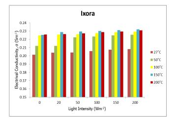
Figure 8 The electrical conductivity for ITO/P3DT/IX Organic solar cell
