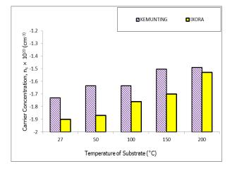
Figure 13 Variation of carrier concentration with temperature of substrate for Bilayer Heterojunction OSCs
