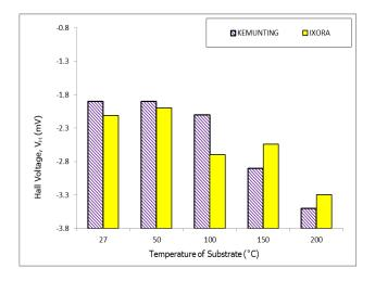
Figure 15 Variation of Hall voltage with temperature of substrate for Bilayer Heterojunction OSCs
