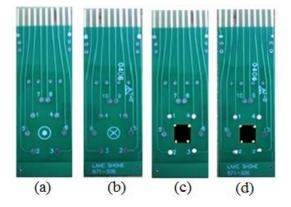
**Figure 6** (a) Back side of sample holder (b) Front side of sample holder (c) Back side of sample holder with mounted samples (d) Front side of sample holder with mounted samples [26]
