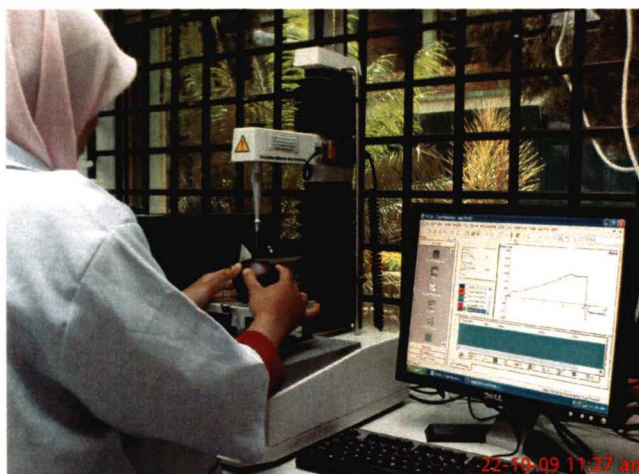
Figure 3.2: Determination of firmness using texture analyzer
