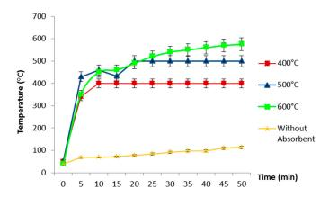
**Figure 2.** Temperature profiles of waste shipping oil during microwave pyrolysis at different temperatures. The data presented are means  $\pm$  SD of three valid runs (*N* = 3) where SD is indicated by the standard deviation bars.
