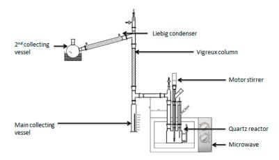
Figure 1. Schematic diagram of microwave pyrolysis apparatus.
