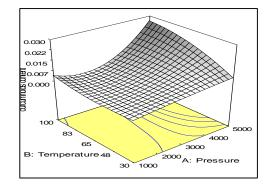
Figure 4 3D-Surface plot of curcuminoid concentration of turmeric oil as a function of pressure and temperature
