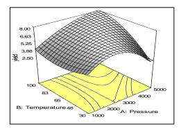
Figure 3 3D-Surface plot of percentage yield of turmeric oil as a function of pressure and temperature
