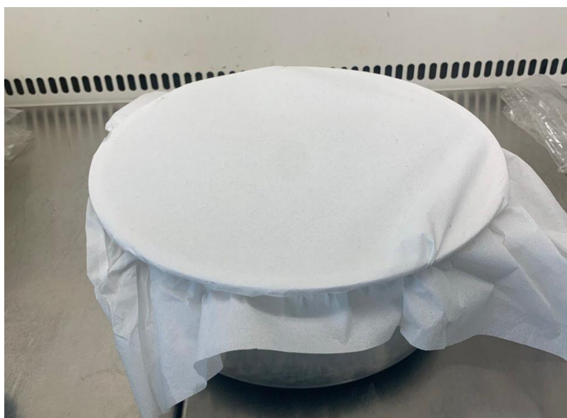
Figure 3.4 Drying process of sporulated solid media after incubation process, covered with triple-folded tissues in a sterile container (Method adapted from Najihah et al., 2021).
