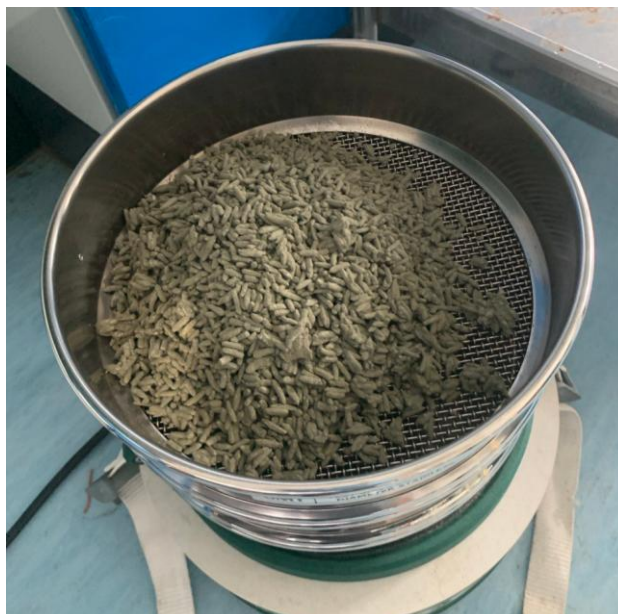
Figure 3.5 Sporulated solid media prior to mechanical harvesting process conducted using two-nested sieve shaker.
