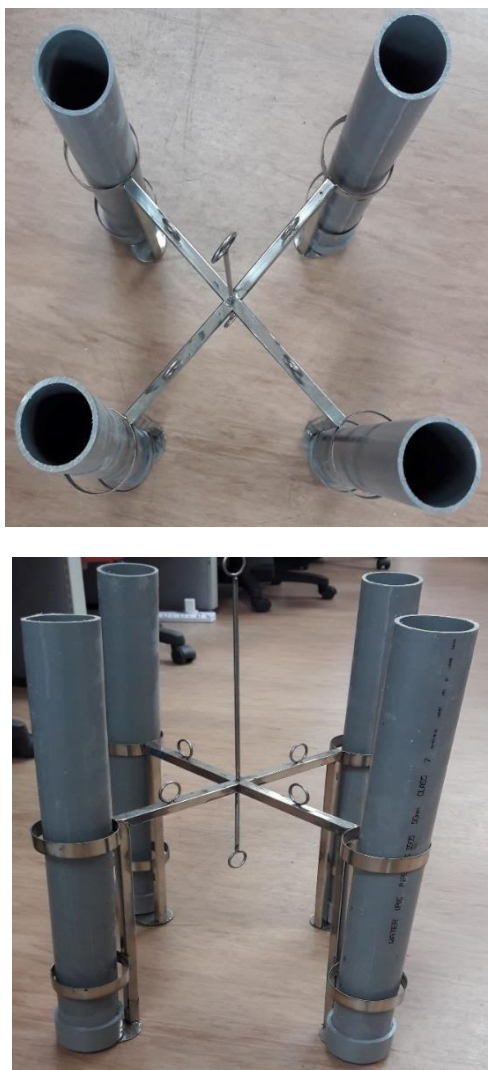
Figure 5.1 The single unit of the trap with four cylinder tubes used for sediment settling experiment.
