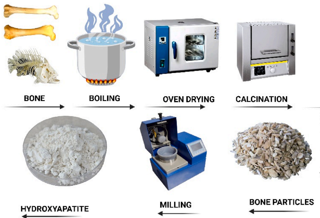
Fig-2. Schematic diagram demonstrating the procedure for the preparation of hydroxyapatite.
